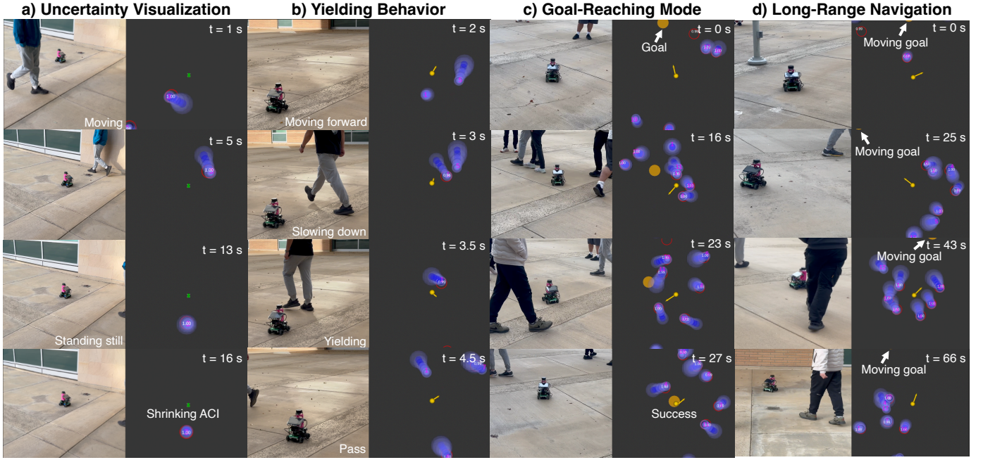
Fig. 5: We deploy our methods on a ROSMASTER X3 with Mecanum wheels using the ROS2 system. For the four subplots, the left sides display photos taken from the experiments, and the right sides show visualizations in RViz. In the RViz visualizations, the red circles represent detection results, and the white numbers inside the red circles indicate the output probabilities of the detection model. The purple numbers correspond to the indices generated by the tracker. The prediction lines are shown in blue, and the prediction uncertainties are depicted in semi-transparent light blue. In (a), the green robot represents the robot’s current location. In (b)-(d), where the decision node is enabled, the yellow sphere indicates the robot’s position, and the yellow arrow represents the command output from the decider node. The orange circle indicates the goal position. (a) In the uncertainty visualization, the human initially walks around the robot and then stands still behind it. The uncertainty area adjusts dynamically based on the prediction accuracy. (b) The robot equipped with Ours (w/ GST) demonstrates stable yielding behavior when interacting with humans. (c) In goal-reaching mode, the robot navigates through crowds and successfully reaches its goal. (d) In long-range navigation mode, the moving goal consistently guides the robot’s movement.
