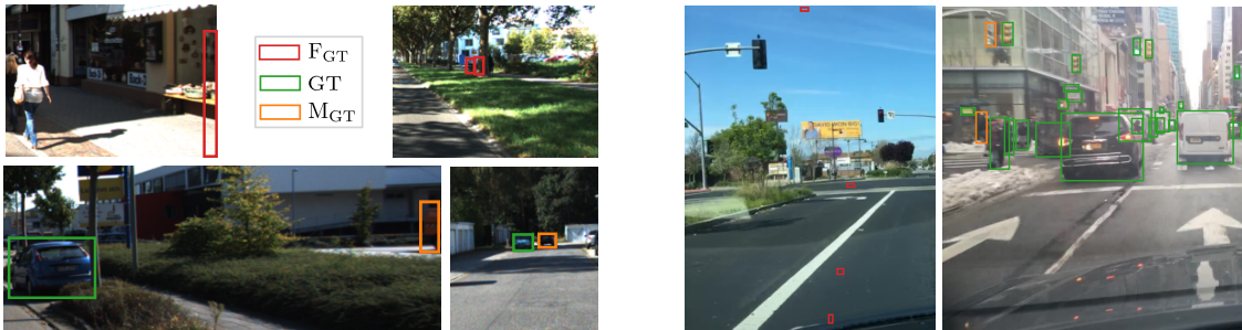
Figure 6: KITTI (left), BDD (right). Examples of GT label errors identified and corrected via our GLC approach. Both human annotators and model-assisted labeling tools often fail to label distant or occluded objects. Moreover, they frequently make errors, such as drawing tiny, incorrect bounding boxes scattered across the images or misplacing boxes near the image edges.
