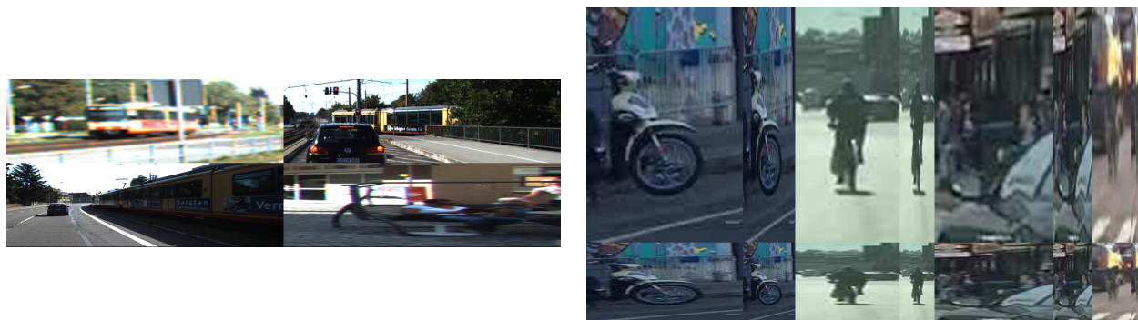
Figure 12: KITTI (left, 4 \times 4 grid setup with \gamma_{r,\min} = 0.5 and \gamma_{r,\max} = 1.0 ), BDD (right, scale variation with \gamma_{r,\min} = 0.25 and \gamma_{r,\max} = 0.75 ). Example collages.
