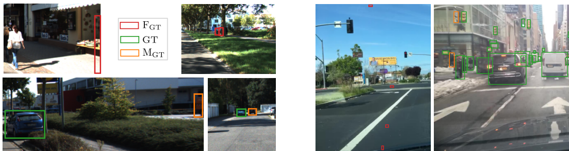
Figure 7: KITTI (left), BDD (right). Examples of GT label errors identified and corrected via our GLC approach. Both human annotators and model-assisted labeling tools often fail to label distant or occluded objects. Moreover, they frequently make errors, such as drawing tiny, incorrect bounding boxes scattered across the images or misplacing boxes near the image edges.
