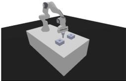
*Peg-in-hole*: the agent controls the Franka arm to perform a peg-insertion task. With two holes available on the desk, the agent can successfully complete the task by inserting the peg into either hole. The episode length is 100.
