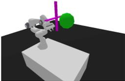
*Reach*: the agent controls the Franka arm to reach the red ball, navigating around a fixed cross-shaped obstacle that lies in the path. Despite the presence of a single goal position, the agent can bypass the obstacle in four distinct ways, offering multiple solutions to the task. The episode length is 100.
