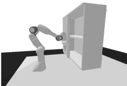
*Cabinet-open*: the agent controls the Franka arm to open a cabinet. The cabinet has two layers therefore the agent can move the arm to either layer and subsequently pull the door open to finish the task. The episode length is 100.
