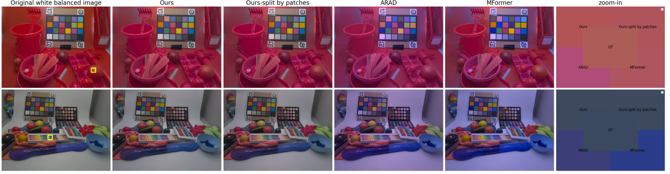
Figure 5. Depiction of the relighting consistency: we input an image to the four networks, relight the prediction, project back to camera RGB and white balance with the new illumination. On the left is the white balanced image under the new illumination. The last column is the RGB value of the projected reconstructions in the marked rectangle in the image.
