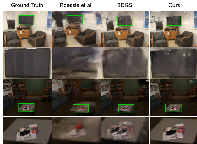
Figure 4: Novel view synthesis results from different methods, namely Roessle et al. [25], 3DGS [14], and our method, on the ScanNet Dataset. With sparse inputs, both [25] and 3DGS struggle to gather enough information to accurately reconstruct challenging areas, such as the television in the first scene. Roessle et al. [25], which uses inaccurate dense prediction for regularization, results in ghost effects and blurring in the rendered images. 3DGS does not employ any regularization and consequently fails to capture some details. In contrast, our method successfully renders a sharper image of the television in the first scene and the books in the second scene.
