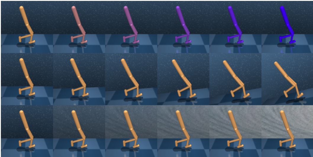
Figure 3: Samples from the modified DistractingCS with intensities increasing from (left-most column) zero to (right-most column) one for the (top row) color, (middle row) camera pose, and (bottom row) background distractions.
