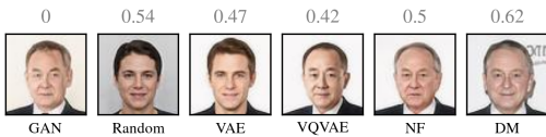
Figure 2. Reconstruction of a CelebA-Synthetic image using various encoders stitched to the GAN decoder. The leftmost image is the ground truth. Stitched models using the VQVAE and NF encoders yield the closest reconstructions.
