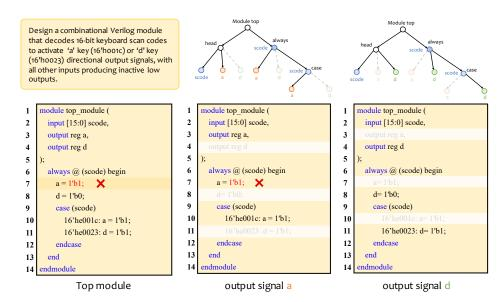
Figure 1: Due to Verilog's characteristics of relatively independent and parallel signals, we can extract the code implementation of a specific signal through AST. Here there are two output signals, we can separately extract their related code implementations. Among them, the implementation of signal a is incorrect while signal d is correctly implemented. We can utilize the code implementation of the correct signal d to provide functional correctness rewards for RL.
