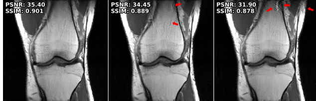
Figure 15: Ablation study on the number of stages for cyclic measurement consistency. Two reconstruction levels (left) outperform deeper variants (middle, right), as additional stages overly rely on synthesized k-space data.
