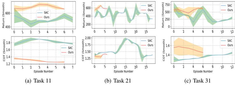
Figure 9: Return (upper) and COT (bottom) of the rapid learning and adaptation process of quadruped robots on new real-world tasks 11, 21 and 31. Task  $MN$  represents the new task number, where  $M$  represents the  $M^{th}$  environment in Figure 8, and  $N$  represents the  $N^{th}$  locomotion target in Table 7. The x-axis represents the number of episodes. The shaded area represents one standard deviation. Each experiment was repeated three times.
