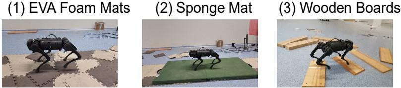
Figure 8: Three new environments are considered in the skill reuse phase of robotic SG, including EVA foam floor mats, sponge mat, and wooden boards respectively.
