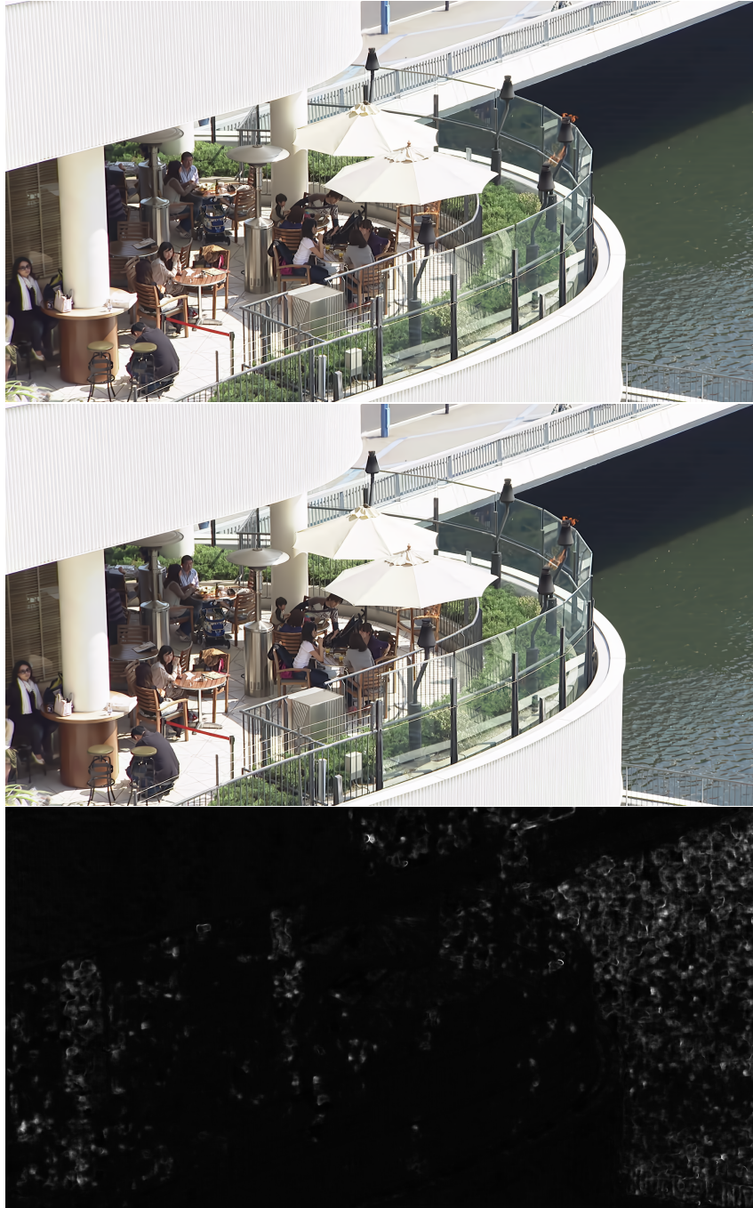
Figure 11: Comparison between our proposed model with DVC Pro on a decoded P-frame from sequence BQTerrace in HEVC B. In this sequence, our proposed model has a bitrate saving of 20.5% over DVC Pro. Top: our proposed model (0.01472 bpp); middle: DVC Pro (0.02587 bpp); bottom: predictive uncertainty.
