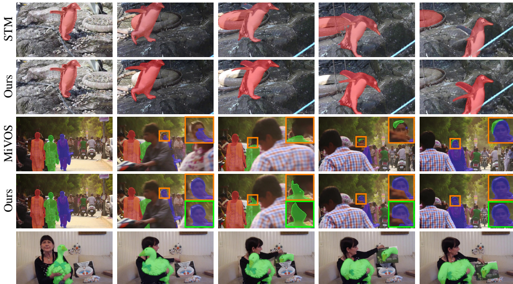
Figure 7: Visualization of semi-supervised VOS results with the first column being the reference masks to be propagated. The first two examples show comparisons of our method with STM [18] and MiVOS [21]. In the second example, zoom-ins inset (orange) are shown with the corresponding ground-truths inset (green) to highlight their differences. The last row shows a failure case: we cannot distinguish the real duck from the duck picture, as no temporal consistency clue is used in our method.
