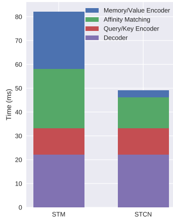
Figure 5: Average running time of each component in STM and STCN.
