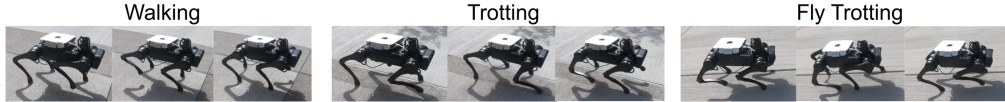
Figure 5: Real world deployment of the learned policy. The robot moves at different speeds with different gaits.
