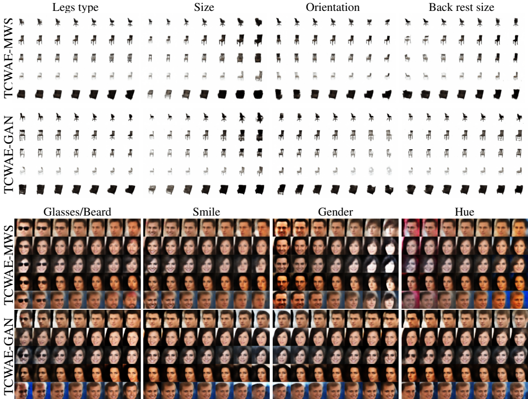
Figure 4: Latent traversals for TCWAE-MWS and TCWAE-GAN. Each line corresponds to one input data point while each subplot corresponds to one latent factor. We vary evenly the encoded latent codes in the interval [-4, 4] .
