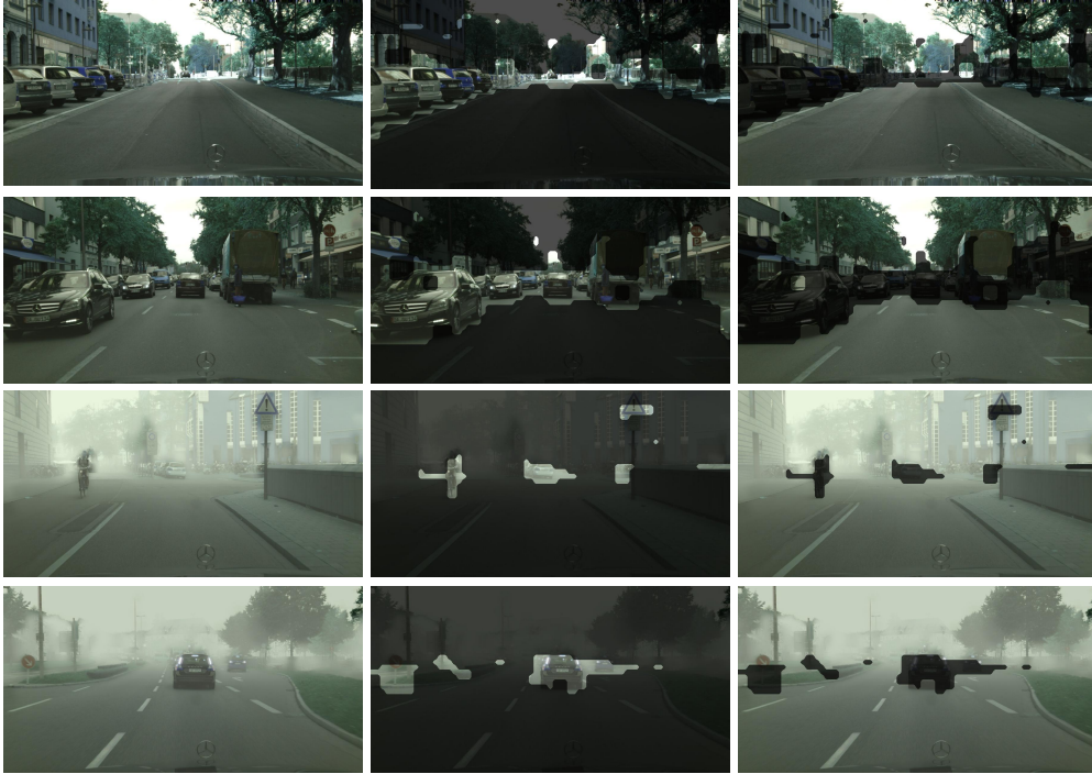
Figure 6: Visualization of gated masks from C→F. The first two rows correspond to the source domain ( i.e. , C) and the last two to the target domain ( i.e. , F). The first column shows the original images, while the last two columns present heatmaps from M_0 and M_1 , where dark regions indicate mask value 0 and others indicate 1.
