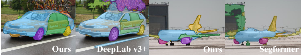
Figure 10: Qualitative results of 2D part segmentation on PartImageNet dataset show that our prediction is more geometry-aware and is less affected by the complex background. Parts are represented by different color masks with highlighted boundaries.
