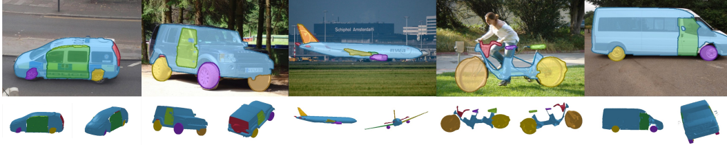
Figure 6: Qualitative results of 3D part recognition from our annotated real images. We show the 2D segmentations and 3D parts rendered from two different views
