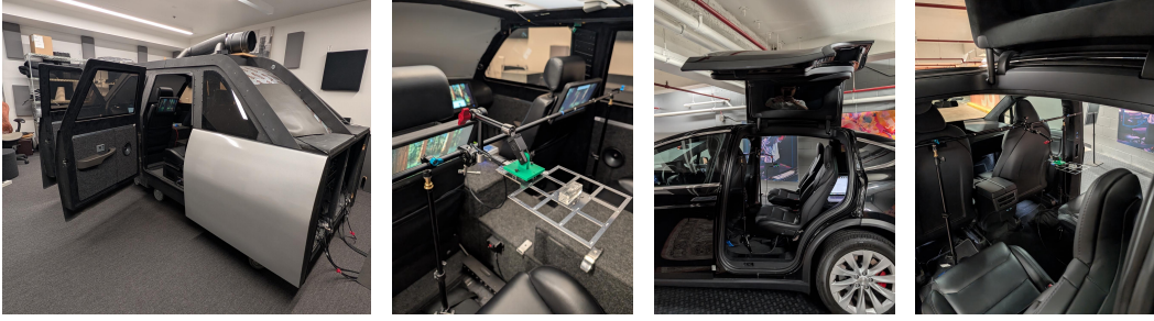
Figure 3: Data collection setup. (a)Left: Data is collected in controlled environment - The BUCK, which is a vehicle mockup with realistic car interior and acoustic frontend. (b)Right: Data is also collected in real environment - Tesla Model X.
