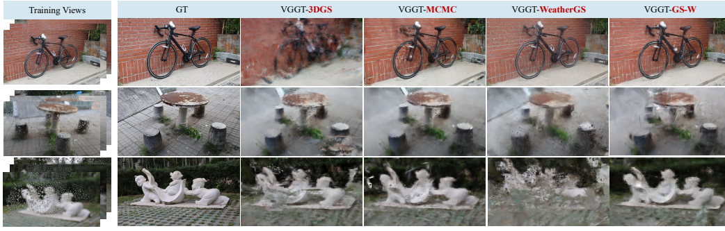
Figure 3: Qualitative Comparison among 3DGS methods: On the raindrop-focused dataset, the original 3DGS loses structural integrity, while GS-W and 3DGS-MCMC retains scene completeness. WeatherGS faithfully reconstructs the scene after raindrop removal but fails to correct background blur. On the background-focused dataset, all methods show moderate performance with artifacts.
