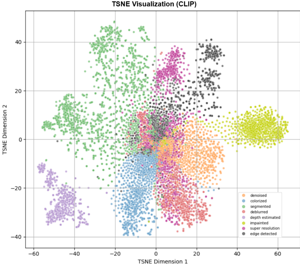
Figure 10: t-SNE Visualization of CLIP-ViT task-specific embeddings. The embeddings represent differences between the transformed image and the original image for each task. CLIP-ViT provides well-separated task clusters.
