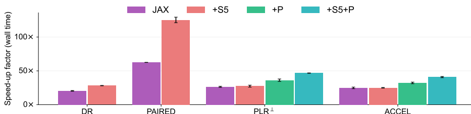
Figure 1: Wall time speed-up factors achieved by minimax relative to PyTorch reference implementations with equal batch sizes (mean and std of 10 runs). Experiments that took 100+ hours now finish in < 3 hours on a single GPU. Here, +S5 indicates the use of an S5 policy, and +P, parallel DCD. (See Section 4 for details.)
