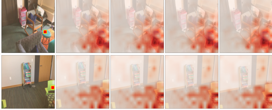
Figure 2: Attention maps from the VoT decoder. Each row shows an original image with a selected query (red square), followed by attention maps from the four subsequent frames. To estimate relative camera pose, VoT attends to the related image regions, resembling the behavior of classical keypoint-based odometry methods.
