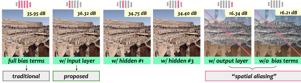
Figure 1: Impact of bias terms in INRs. Pink and Ashen in the top row indicate layers with and without bias terms, respectively. Applying bias terms (without gradient propagation 2 ) to the input layer achieves optimal performance, while lacking bias terms or only applying them to output layer results in “spatial aliasing” manifested as central symmetry in failed reconstructions.
