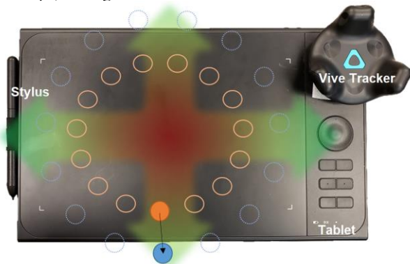
Figure 2: Overlay of Fitts' law task on the tablet. Orange circles depict the physical target location, while blue circles depict the targets the user saw in VR. Gradient arrows illustrate the surface warping effect and how the virtual surface grows in size in all directions.
