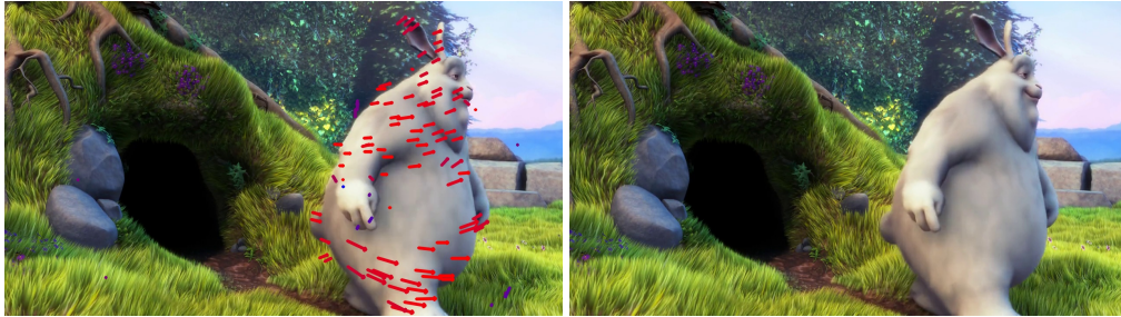
Figure 1: Illustration of motion vectors. The top figure is a snapshot from Roosendaal (2008) including a sub-sample of the motion vectors computed to the next frame (blue color corresponds to movement to the left and red corresponds to movement to the right), which is included below. Observe that while the most of vectors follow the movement, there is noise in the directions (either in magnitude or the direction of the moment) as evidenced by the small vector on a rock and a grass leaf in the left half of the image.
