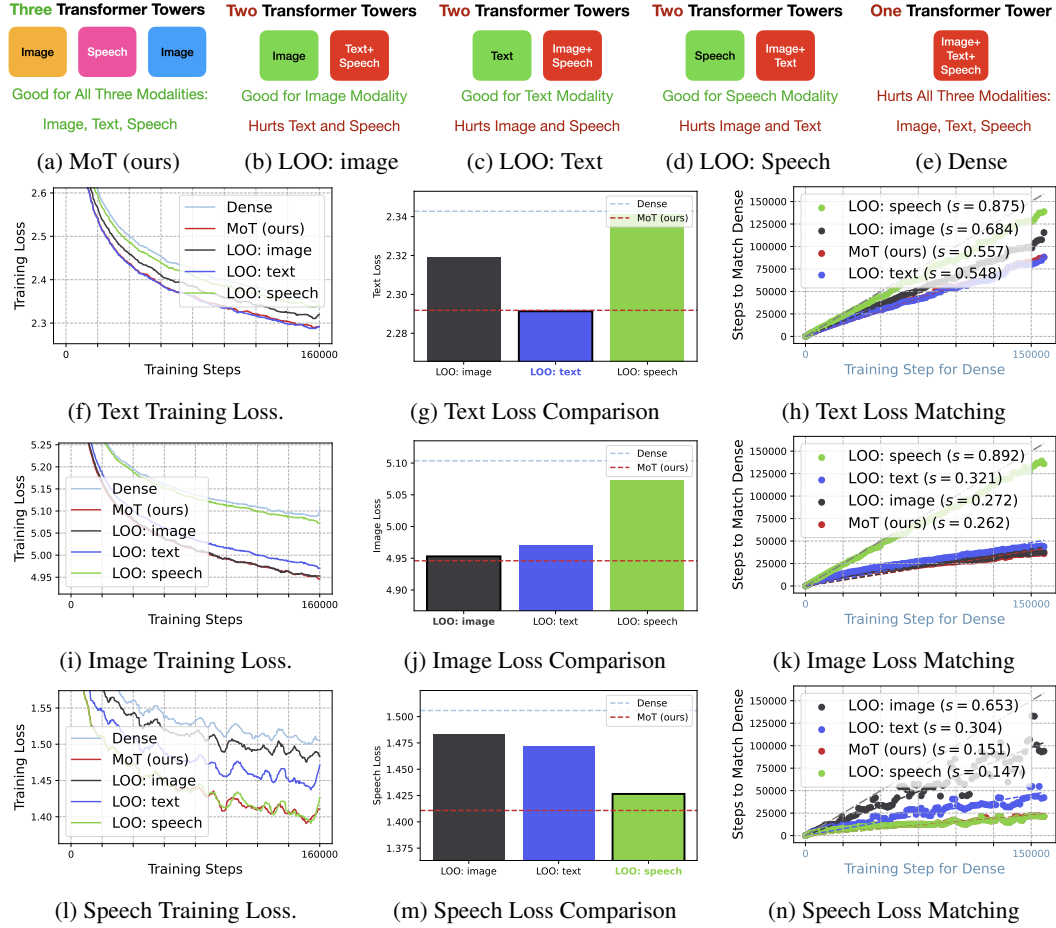
Figure 15: Modality Leave-One-Out (LOO) analysis of MoT variants in Chameleon+Speech setup. a , Proposed MoT architecture with separate transformer towers for image, text, and speech. b-d , Two-tower MoT variants for three modalities: b , Text and speech combined (LOO: image). c , Image and speech combined (LOO: text). d , Text and image combined (LOO: speech). e , Dense transformer with single tower for all modalities. All models ( a-e ) have equivalent FLOPs. f-n , Performance results across modalities. Combining modalities in a single tower consistently degrades performance, while separation improves results. LOO: text, LOO: image, and LOO: speech achieve lowest losses in their respective isolated modalities ( g,j,m ). Analysis highlights the importance of modality-specific parameter allocation for optimal performance. All models are 443M in size. For sparse models, size indicates activated parameters. All runs are FLOPs-controlled and pre-trained from scratch.
