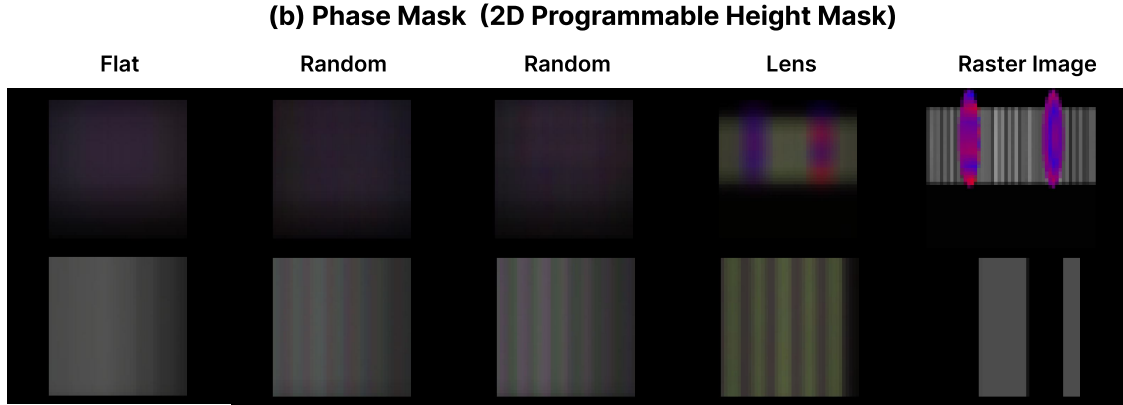
Fig. B7: Sampling optical elements in the Optical Gene: We illustrate examples of sampled optical elements (phase masks) within the Optical Gene for Detection (top row) and Navigation (bottom row) tasks. The figure shows Flat, and 2 Randomly samples phase masks which shows the complexity of the design space. These visualizations also demonstrate that while using a lens is a major innovation in eye design, creating a focused lens is a hard problem that evolution solved really well.
