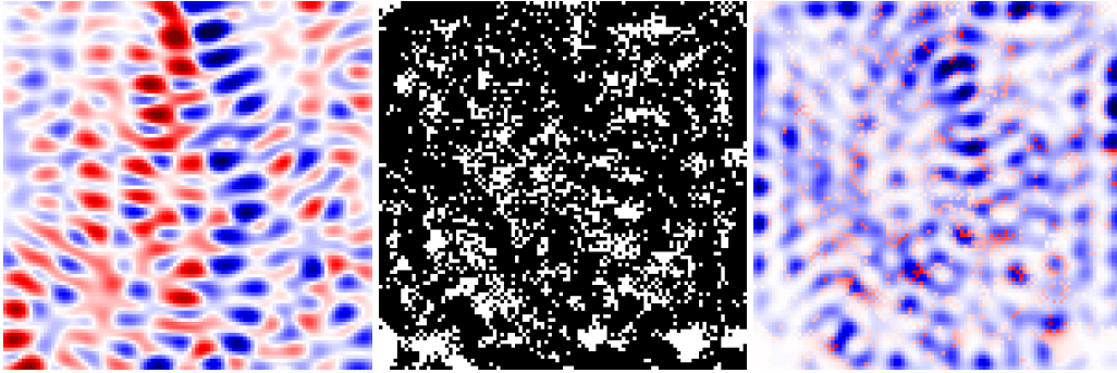
Figure A.9: Left: R_t \odot S_t at t = 0 , i.e., for all-material state. Mid: Local fitness maximum obtained via SA. State S_t at t = t_{max} . Right: R_t \odot S_t at t = t_{max} . Even though initial distribution was clustered, isolated pixels of SA states cause breaking of clustered structure and thus no clusters occur in final state.
