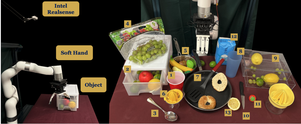
Figure 4: Left: Workspace Setup. We place an Intel Realsense camera above the robot to maintain an egocentric viewpoint, consistent with the affordance model’s training data. Right: Thirteen objects used in our experiments.
