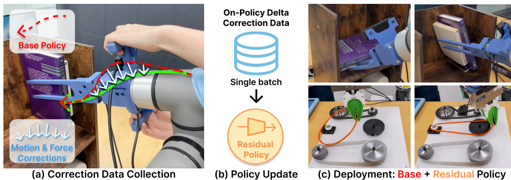
Figure 1: CR-DAGger . To improve a robot manipulation policy, we propose a compliant intervention interface (a) for collecting human correction data, and use this data to update a compliant residual policy (b), and thoroughly study their effects by deploying the updated policy on two contact-rich manipulation tasks in the real world (c).
