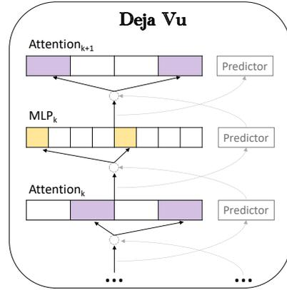
Figure 2. DEJAVU uses lookahead predictors to side-step prediction costs: given the input to the attention layer at block  $k$ , they (asynchronously) predict the contextual sparsity for the MLP at block  $k$ , and given the input to the MLP at block  $k$ , they predict the sparsity for the attention head at the next layer.
