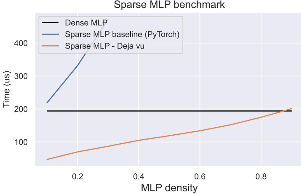
Figure 13. Speed benchmarking of the MLP layer of OPT-175B on 8xA100s. Our sparse implementation is up to  $4.5\times$  faster than the baseline implementation in PyTorch. Our sparse MLP implementation remains faster than dense MLP for density up to 0.8.
