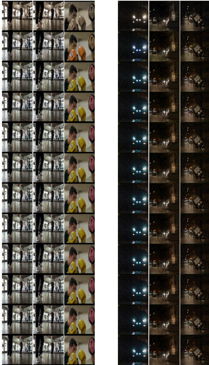
Figure 12: Some samples from the MCL-JCV Wang et al. (2016) dataset. The columns represent different frames, while the rows display progressively improving levels of quality from top to bottom, produced by MCUCoder.
