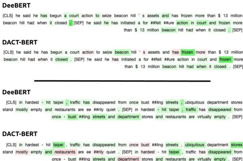
Figure 3: Output prediction attribution to each input token. Two samples from the MRPC task are shown with their attributions obtained both for DeeBERT and DACT-BERT. The color intensity shows the degree on how much each token contributes to the final output. Green is used for tokens that have positive attribution to the output, while red means tokens with negative attribution to the output.
