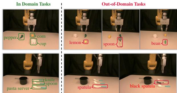
Fig. 4: Real-world generalization experiments. In-Domain and Out-of-Domain settings in the real world on a FANUC LRMate 200iD/7L robotic arm.
