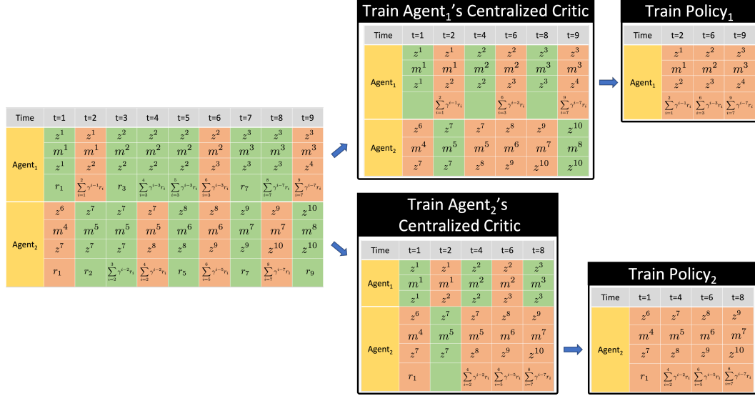
Figure 8: An example of the trajectory squeezing process in Mac-IAICC: each agent learns an individual centralized critic for the decentralized policy optimization. In order to achieve a better use of centralized information, the recurrent layer in each critic’s neural network should receive all the valid joint macro-observation-action information (when any agent terminates its macro-action (line 20-22) and obtain a new joint macro-observation). However, the critic’s TD updates and the policy’s updates still rely on each agent’s individual macro-action termination and the accumulative reward at the corresponding timestep (line 23-26). Hence, the trajectory squeezing process for training each critic still depends on joint-macro-action termination but only retaining the accumulative rewards w.r.t. the corresponding agent’s macro-action termination for computing the TD loss (the middle part in the above picture). Then, each agent’s trajectory is further squeezed depending on its macro-action termination to update the decentralized policy.
