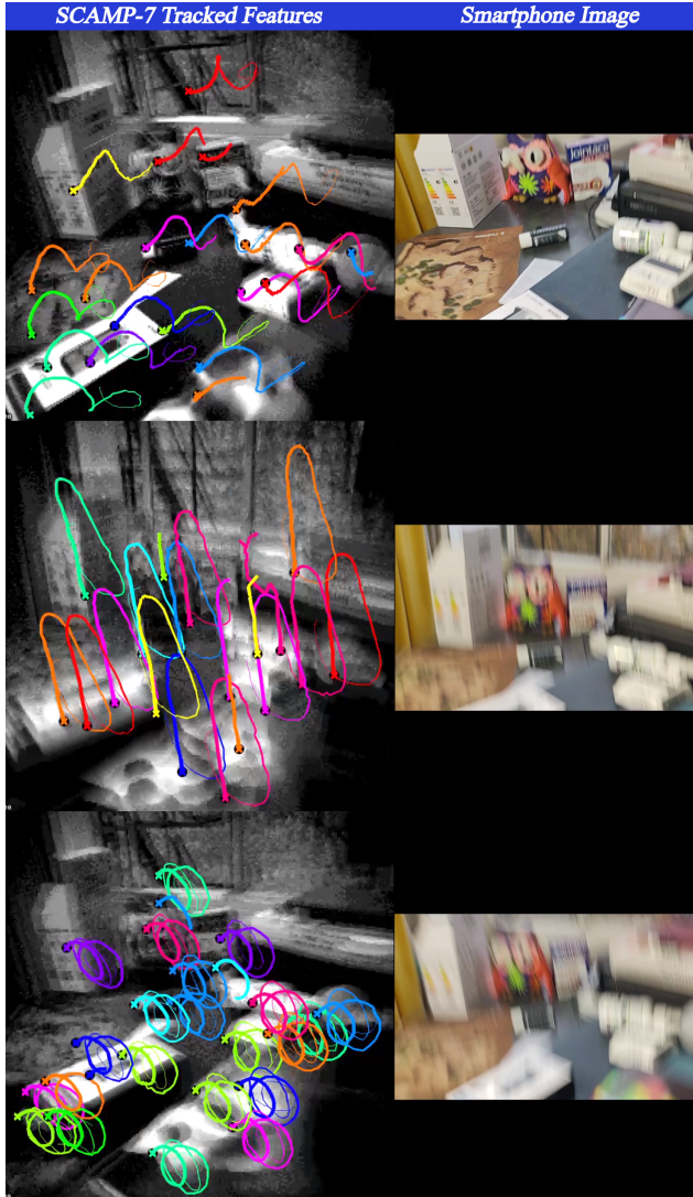
Figure 7. Examples of feature tracking on SCAMP-7. Left Column: Trails of point-features tracked by SCAMP-7, with thickness representing age. Right Column: 60 FPS video from smartphone mounted alongside SCAMP-7. Our approach tracks features reliably under motion that renders the smartphone’s image near unusable. Here SCAMP-7 also outputs an image temporally ( 1/16^{th} per frame) for visualization, limiting performance to around 850 FPS. The motion blur in SCAMP-7 images shown is an artefact of this image readout scheme, and is not present internally.
