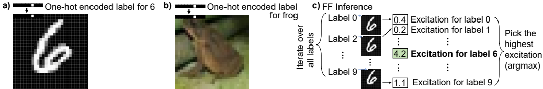
Figure 1: a) Label embedding into an example MNIST image. b) Label embedding into an example CIFAR10 image. c) FF inference iterates over all possible labels in the dataset.
