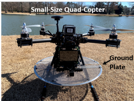
Figure 2: The UAV equipped with u-blox GPS receiver and multispectral camera
