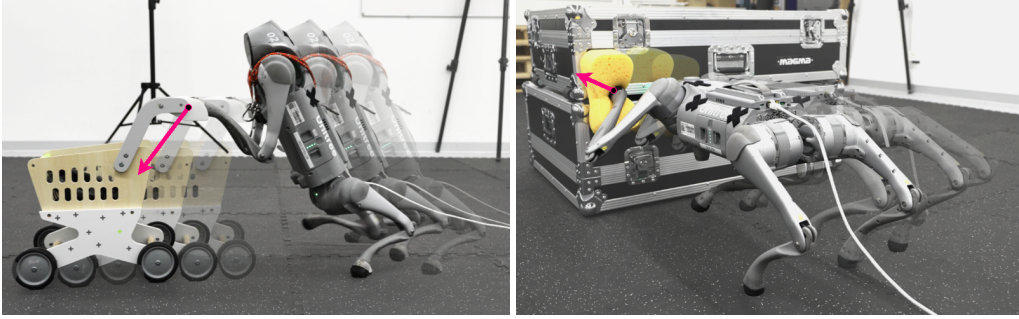
Figure 3: Snapshots of two whole-body loco-manipulation tasks, where the desired EE force are overlaid as pink arrows. Upper : pushing a shopping cart while walking in bipedal mode; bottom : holding a sponge while walking in quadrupedal mode.
