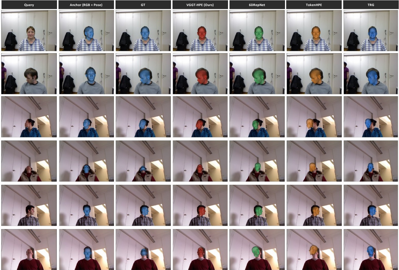
Figure 4. Qualitative results on BIWI. Each row shows a different subject. From left to right: the query frame, the anchor frame with its known pose overlay, the ground-truth pose, our prediction (VGGT-HPE), and three baselines (6DRepNet, TokenHPE, TRG). Our method produces pose estimates that are visually closer to the ground truth across a range of head orientations, including challenging near-profile and upward-looking poses where absolute methods exhibit larger deviations.
