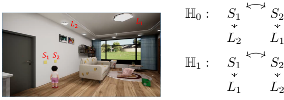
Figure 4. The simulation environment for the switch-light reasoning task. The agent is required to identify which switch ( S_1 and S_2 ) controls which light ( L_1 and L_2 ) through active exploration. The causal graphs under \mathbb{H}_0 and \mathbb{H}_1 are shown on the right.
