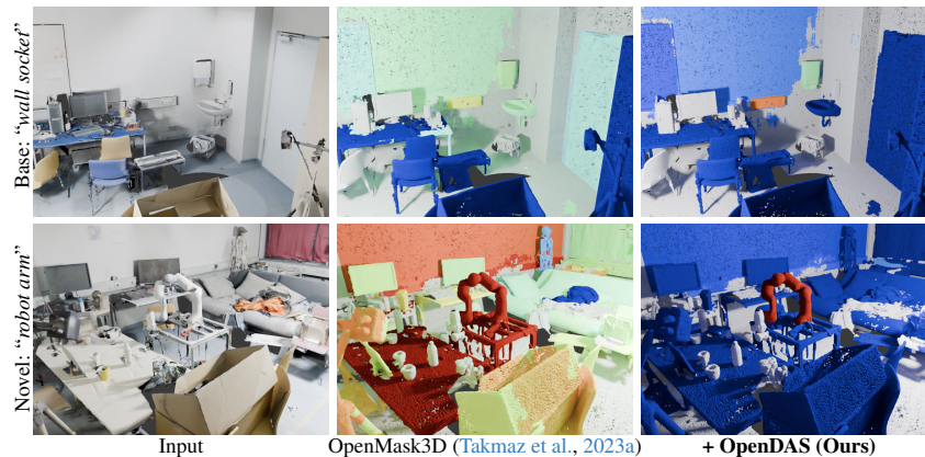
Figure 6: Qualitative Results on Open-Vocabulary 3D Instance Segmentation. We show the query-response scores of OpenMask3D (Takmaz et al., 2023a) predicted with CLIP (Radford et al., 2021) and our OpenDAS. Blue indicates low similarity with the text query and red high similarity. Unlike CLIP, our OpenDAS can better localize the correct mask with a higher similarity score.
