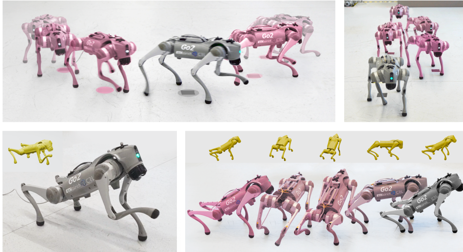
Figure 8: Hardware deployment of RobotKeyframing for position targets ( top ), and full-pose targets ( bottom ). Posture keyframes are displayed in yellow.
