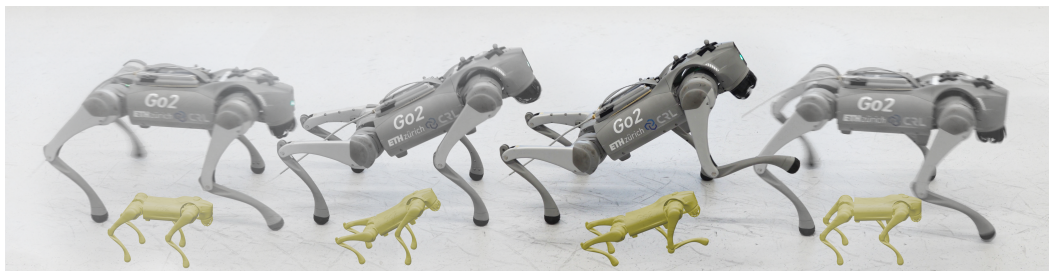
Figure 1: RobotKeyframing : Locomotion policy trained with our framework meets the keyframes with position and full posture targets (yellow) at specified times on hardware experiments.
