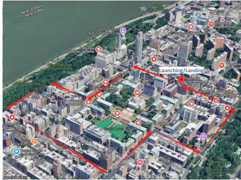
Figure 2: Urban layout and flight path for the cruising scenario. The UAV departs from the Mudd building (red point), follows the red path through streets and courtyards to the riverside, circles the campus, and returns.
