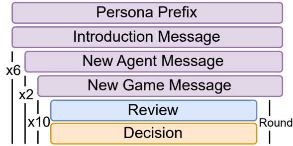
Figure 7: The data collection pipeline of a single LLM-based player. The player is initialized with a prompt that contains the persona prefix followed by the introduction message. Then, nature (purple) manages the conversation between the agent (blue) and the LLM-based player (orange). Practically, the LLM-Chat agent receives a concatenation of all purple and blue parts sent since its last message as a single message.
