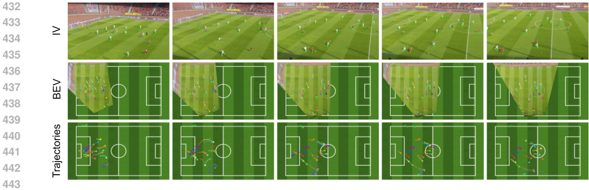
Figure 6: We showcase the results of applying our technique on soccer video clips. We demonstrate the players’ localization results in the image view (IV) on the first row and BEV as well on the second row as the corresponding trajectories on the bottom row.
