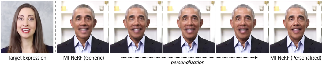
Figure 7: Progressive personalization from our generic MI-NeRF trained on 100 identities to the personalized model for a target identity.
