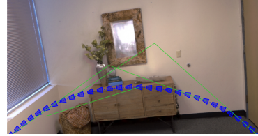
Figure 3: The blue curve represents the optimized camera trajectory as selected keyframe poses.
