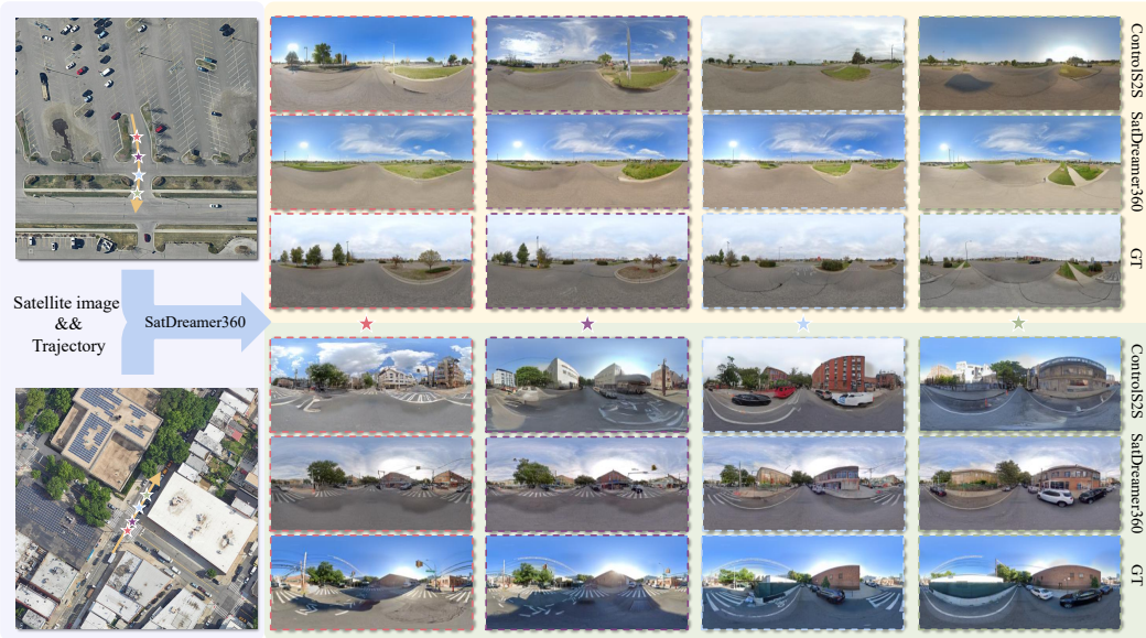
Figure 1: Given a satellite image and a sequence of query poses (colored stars), our goal is to synthesize coherent panoramic views along the trajectory. The proposed SatDreamer360 generates more realistic and geometrically consistent ground-level scenes compared to state-of-the-art methods, faithfully capturing spatial layouts and structural continuity across diverse environments.
