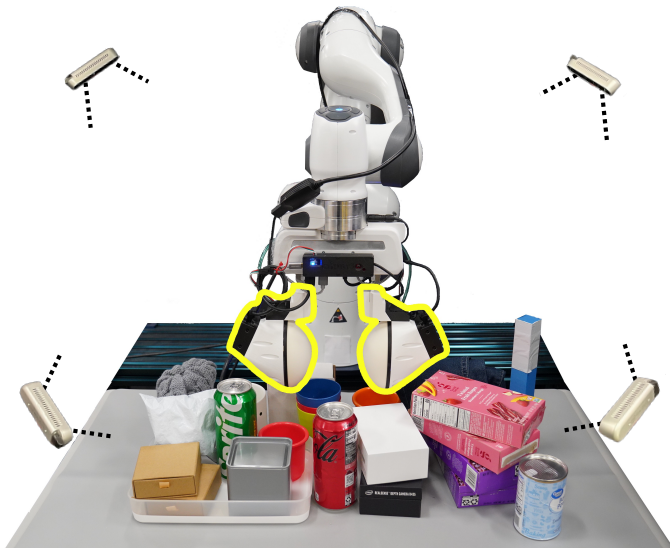
Fig. 6: Hardware overview. Our experimental platform consists of a Franka Panda arm, two Soft-Bubble grippers, four RealSense D415 RGBD cameras, and a diverse set of objects.
