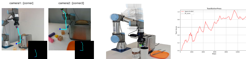
Figure 16: Training curves of the real-world ToastButtonPress task, where the environment is cluttered
